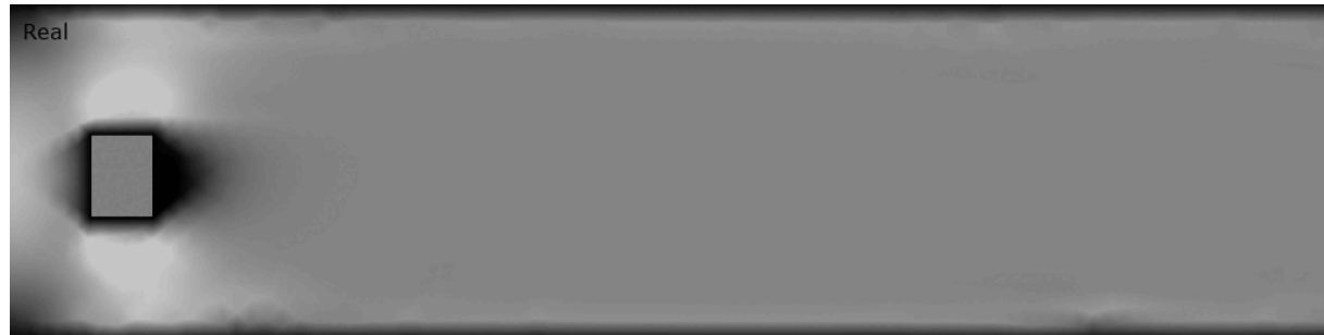
Numerical simulation of the vortex street behind a rectangular obstacle.
